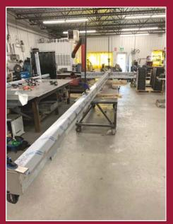
New stainless steel cladding, as well as jointing welds and details make our cross more substantial than the original.
